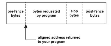
This figure shows the layout of heap debugger overhead in a block. The pre-fence, slop, and post-fence are optional. See "slop=n" on page 7-55.
