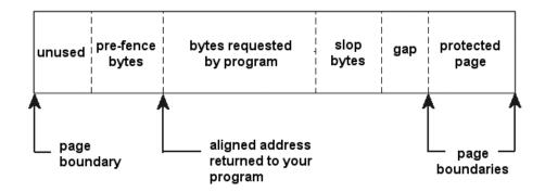
This figure shows the layout of heap debugger overhead in a block with hardware overrun protection. The pre-fence and slop are optional. See "slop=n" on page 7-55. The gap may be zero sized; otherwise it typically is filled with the post-fence fill byte.
