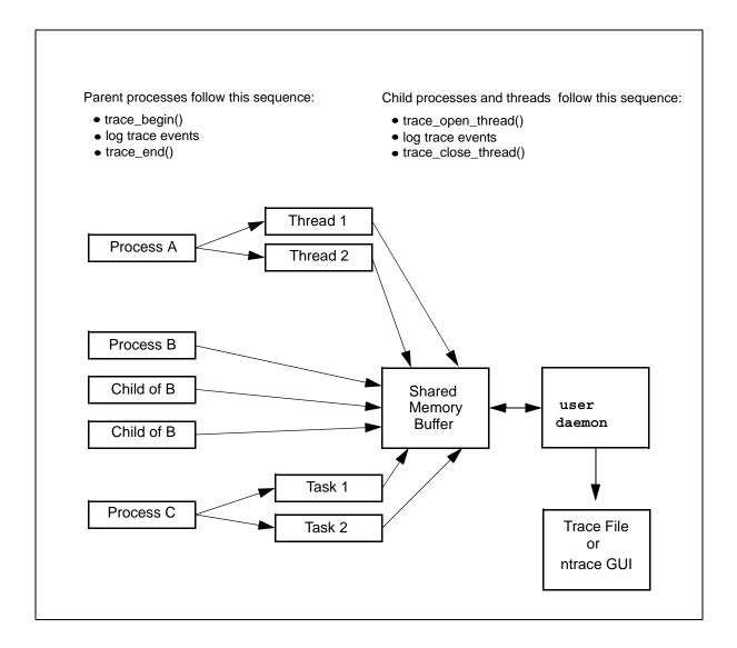
Figure 2-1. Inter-Process Communication and Library Routines
