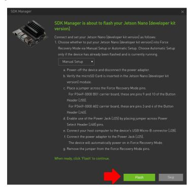
Follow the steps listed on the Flash dialog to place the Jetson Nano into recovery mode and then click the Flash button to begin flashing.
