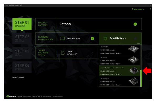
2. Click on the Jetson Nano (Developer Kit Version) target hardware option to make it the selected target, as shown in the following screenshot:
