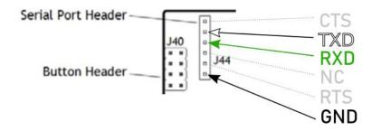
• To connect the USB serial cable, attach the White wire to TXD, the Green wire to RXD and the Black wire to GND as shown in the following picture:
