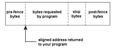
This figure shows the layout of heap debugger overhead in a block. The pre-fence, slop, and post-fence are optional. See "slop=n" on page 6-58.
