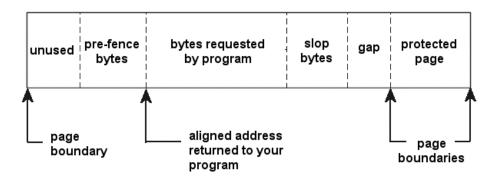
This figure shows the layout of heap debugger overhead in a block with hardware overrun protection. The pre-fence and slop are optional. See "slop=n" on page 6-58. The gap may be zero sized; otherwise it typically is filled with the post-fence fill byte.
