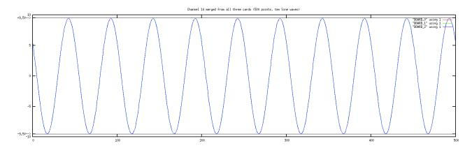
The following plot contains 500 sample points of channel 16 from all three cards. You should see ten Square waves from each of the three cards, and these wave should overlap if the clocks on all three cards are properly synchronized
