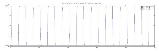
The following plot contains 250 sample points of channel 14 & 16 from all three cards. You should see five Sine and five Square waves from each of the three cards, and these wave should overlap if the clocks on all three cards are properly synchronized
