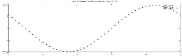
The following plot contains 50 sample points of channel 16 from all three cards. You should see a single Square wave from each of the three cards, and these wave points should overlap if the clocks on all three cards are properly synchronized
