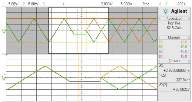
The above displays two channels (Ch0-yellow and Ch32-green) generating a triangle wave at 100Hz. Now, the user performs the phase change request, however, this time setting the *immediate* value to
