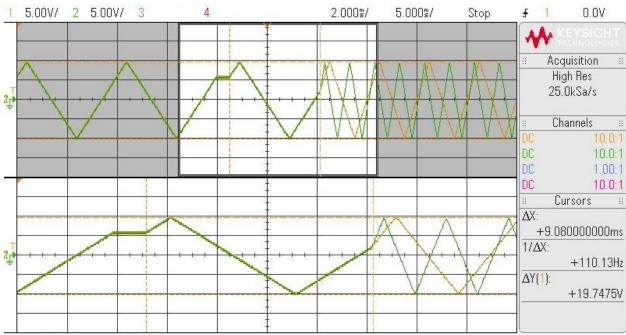
This time, we are demonstrating a smart-seamless transition of two channels. The operation is the same as Seamless Operation but the distance from the end of the flat line (when the clock is restarted) to the point where the two waves change frequency shows approximately 10ms. The smart seamless operation
