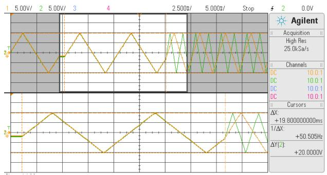
This time, we are demonstrating a seamless transition of two channels. Here, both Ch0 and Ch31 are generating a triangle wave at 100Hz. The frequency is then changed seamlessly where Ch0 is changed to 200Hz (yellow) and Ch31(green) is changed to 400Hz. Also, a temporary "hook" was placed in the test program to stop/start the system clock just prior to calling the change *frequency* API. The reason is to
