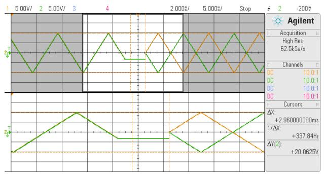
The above displays two channels (Ch0-yellow and Ch32-green) generating a triangle wave at 100Hz. Now, the user performs the phase change request, however, this time setting the *immediate* value to
