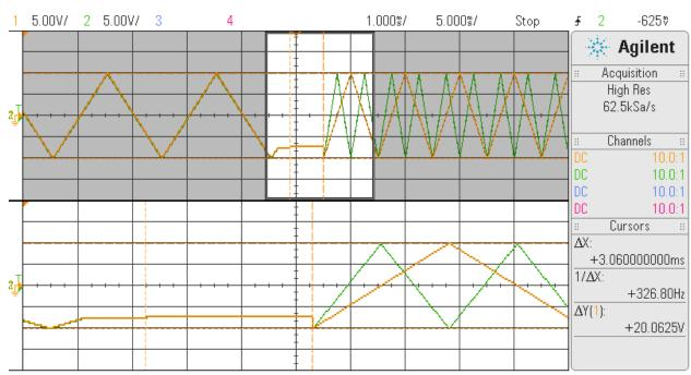
The above displays two channels (Ch0-yellow and Ch32-green) generating a triangle wave at 100Hz. Now, the user performs the frequency change request, however, this time setting the *immediate* value to '1'. Once again, the test was modified to stop/start the clock and hence the timing from the re-starting of the clock to the restarting of the waves is approximately 3ms. This time basically represents the partial
