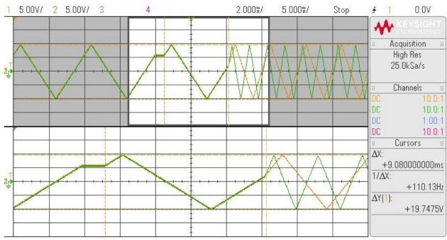
This time, we are demonstrating a smart-seamless transition of two channels. The operation is the same as Seamless Operation but the distance from the end of the flat line (when the clock is restarted) to the point where the two waves change frequency shows approximately 10ms. The smart seamless operation is capable of reducing the latency by keeping track of the current position of the Multiplexor buffers and only keeping the minimum amount of samples to provide a seamless transition.
