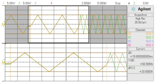
This time, we are demonstrating a seamless transition of two channels. Here, both Ch0 and Ch31 are generating a triangle wave at 100Hz. The frequency is then changed *seamlessly* where Ch0 is changed to 200Hz (yellow) and Ch31(green) is changed to 400Hz. Also, a temporary "hook" was placed in the test *Concurrent Real-Time™ ccuraocc-wave Library for RedHawk Linux™ – Release Notes* - 10 -
