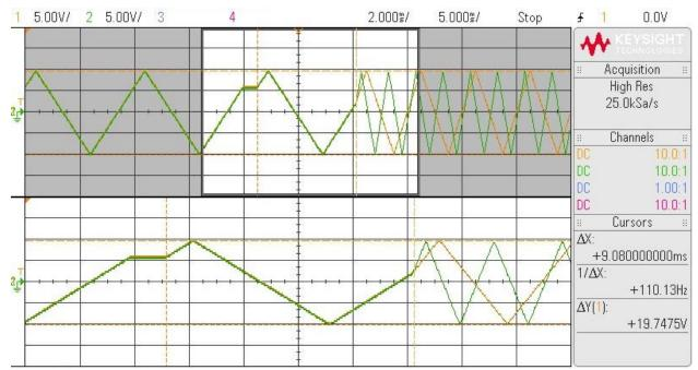
This time, we are demonstrating a smart-seamless transition of two channels. The operation is the same as Seamless Operation but the distance from the end of the flat line (when the clock is restarted) to the point where the two waves change frequency shows approximately 10ms. The smart seamless operation is capable of reducing the latency by keeping track of the current position of the Multiplexor buffers and only keeping the minimum amount of samples to provide a seamless transition.
