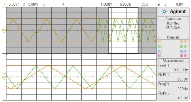
Same wave run as above, however, showing the changed waves. As seen on the right under Measurement, the changed frequency of the two waves is shown by the scope.
