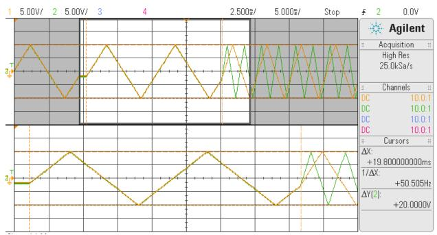
This time, we are demonstrating a seamless transition of two channels. Here, both Ch0 and Ch31 are generating a triangle wave at 100Hz. The frequency is then changed *seamlessly* where Ch0 is changed to 200Hz (yellow) and Ch31(green) is changed to 400Hz. Also, a temporary "hook" was placed in the test Concurrent Real-Time™ ccuraocc-wave Library for RedHawk Linux™ − Release Notes - 10 -
