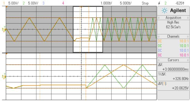
The above displays two channels (Ch0-yellow and Ch32-green) generating a triangle wave at 100Hz. Now, the user performs the frequency change request, however, this time setting the *immediate* value to '1'. Once again, the test was modified to stop/start the clock and hence the timing from the re-starting of
