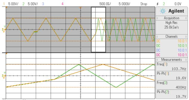
Same wave run as above, however, zooming into the region where the wave change is occurring from 100Hz to 200Hz (Ch0-yellow) and 400Hz (Ch31-green).
