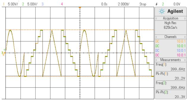
Two waves (Ch0 - yellow & Ch31 - green) displayed above using the wave generation. They were both started at the same time and running at the same frequency of 400 Hz. They are placed one on top of the other to show that they are in phase. During this run, all 32 channels were running the same wave at 400KSPS.
