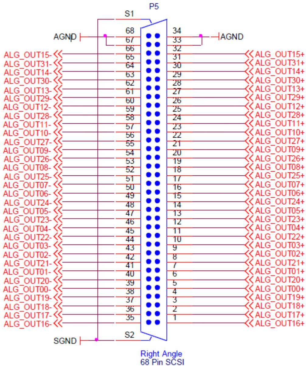
>>>An analog ground connection is always required for the ESD and over/under voltage protection circuits to function correctly.
