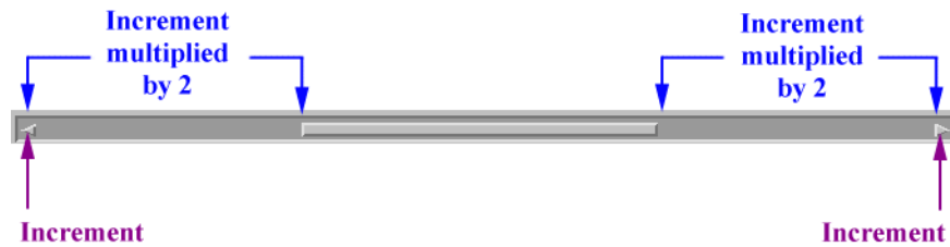
Figure 7-7. Amount of Scrolling Due to Increment Value
