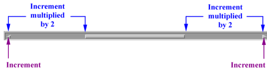
Figure 8-13. Amount of Scrolling Due to Increment Value
