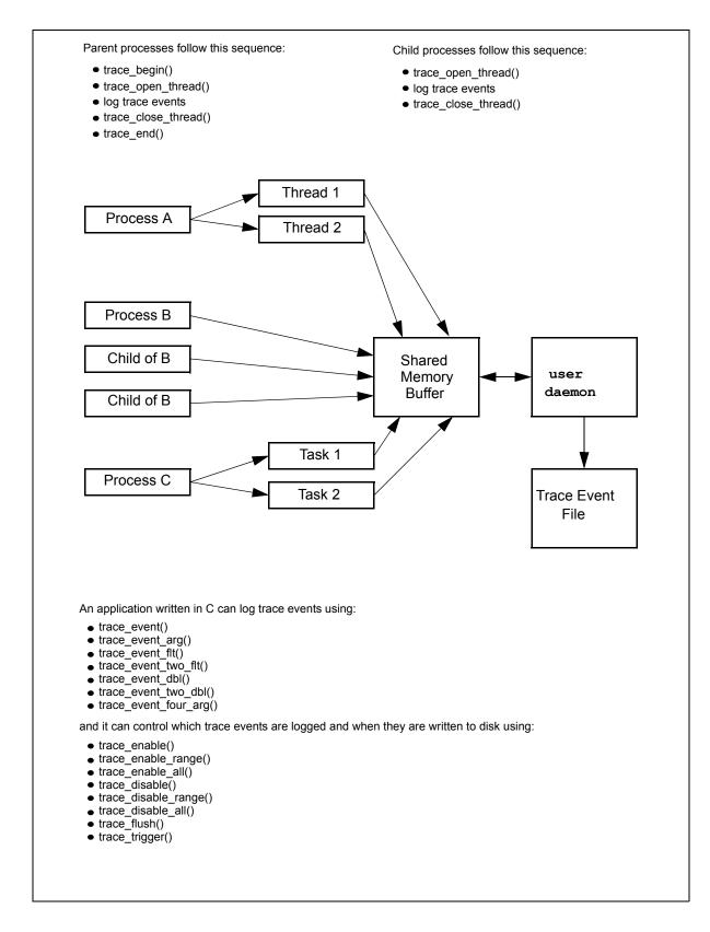
Figure 2-1. Inter-Process Communication and Library Routines
